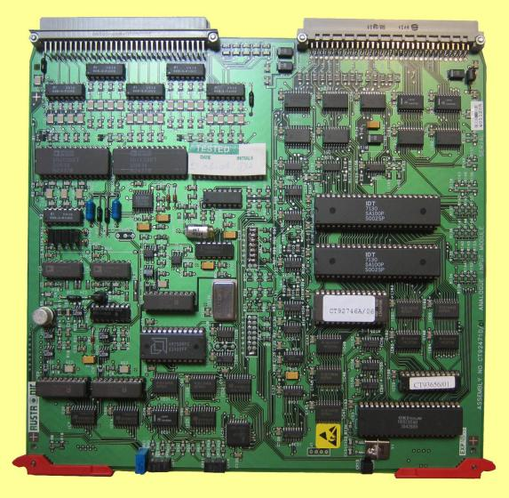
The circuit modules each plug into two electrical connections at the chassis, the lower row of connectors from an industrial standard G64 bus, the upper connects provides input-output connections.
